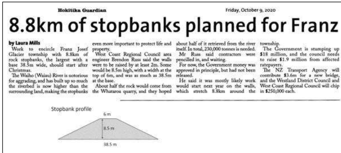
Fig. 4 Information and cross-section of planned stopbanks (Hokitika Guardian, 2020)
